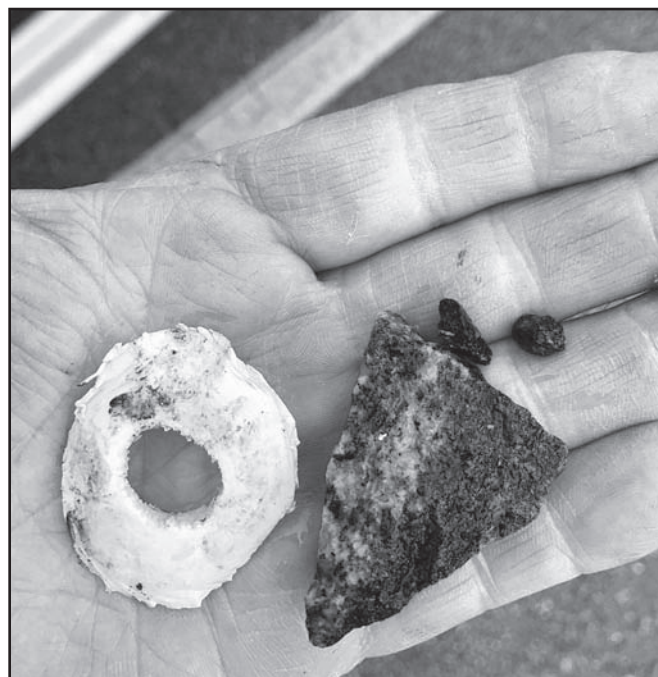
Regular flushing is important in order to clear debris that may collect in the water lines leading to the city's hydrants.
